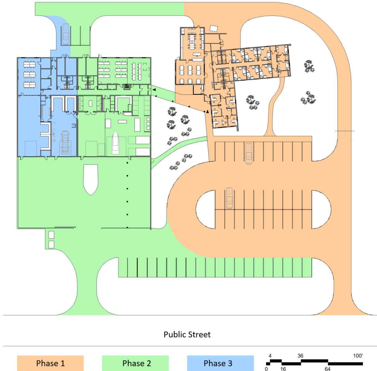
Figure 5: New Facility Phasing Summary.
