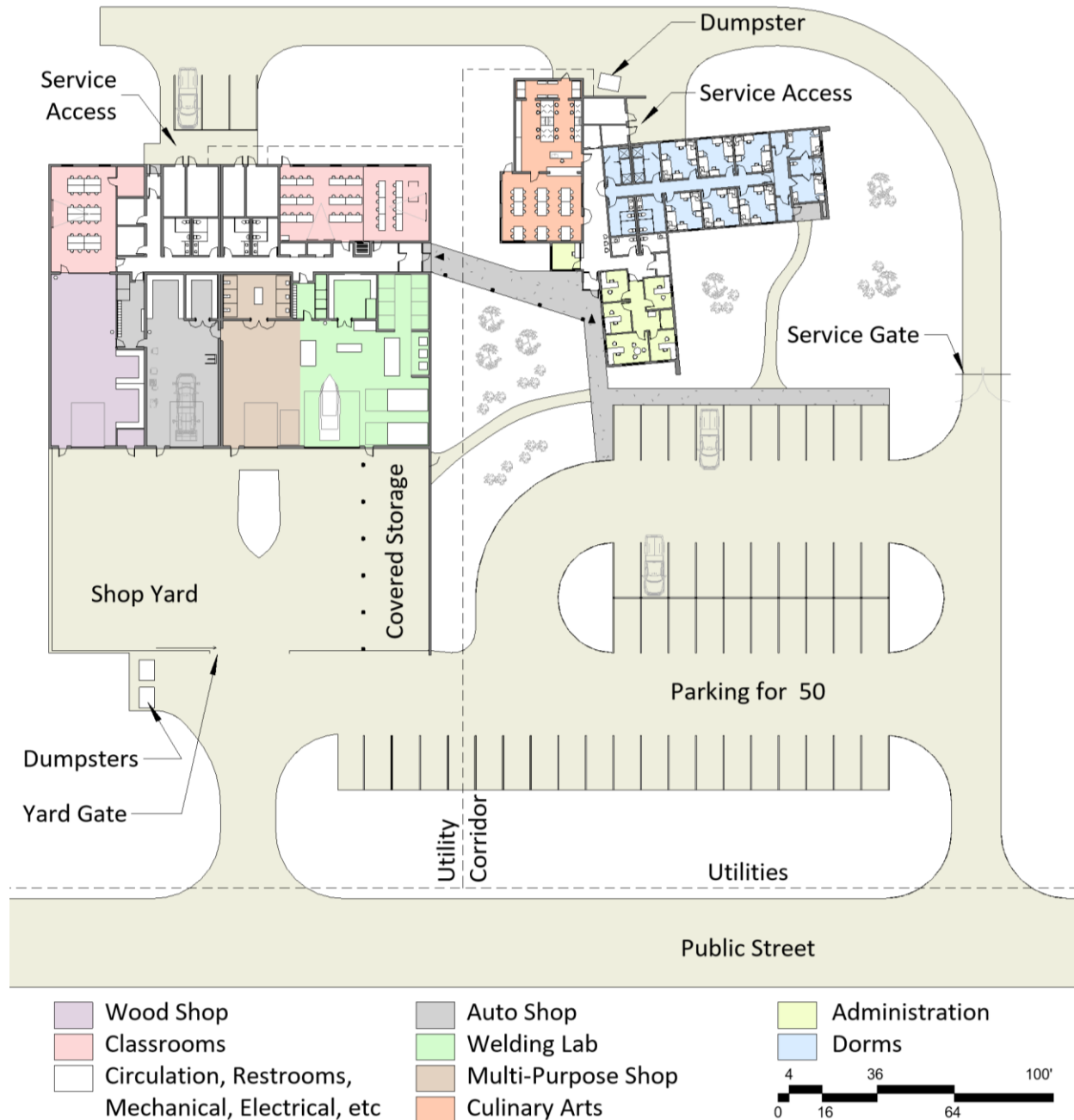
Figure 3: Overall Site Plan for SAVEC Facility.
